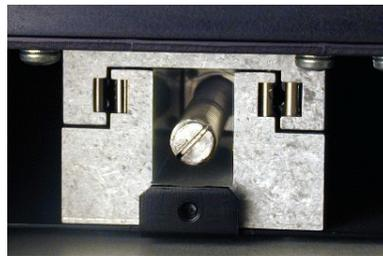
7. Put a small amount of the TEFLON LUBRICANT on the head of a flat head screwdriver and apply it to the screw shaft inside the housing near the other end where the shaft goes into the bearing.
